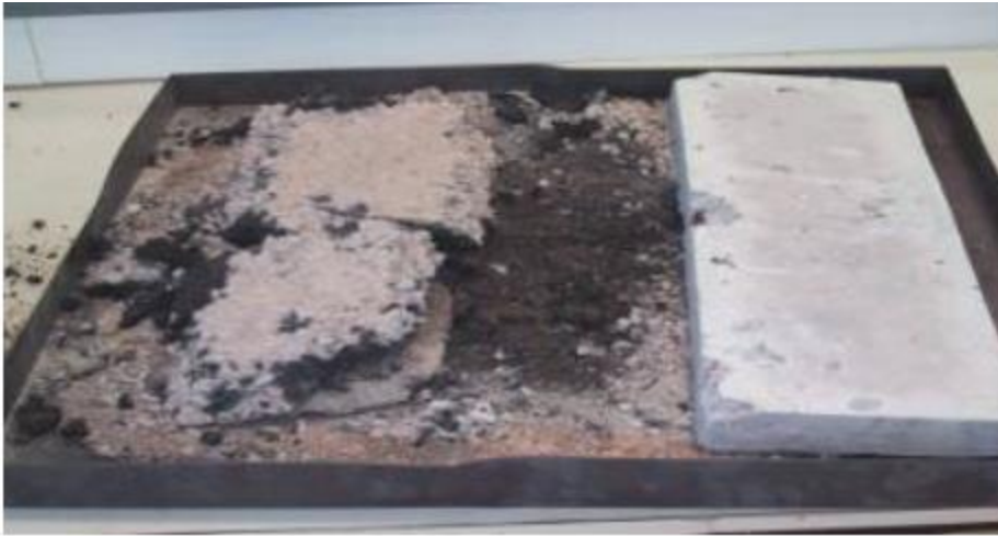
Figure 2. Asphalt (left) and concrete (right) exposed to 750°C (1382°F) heating experiment from (Rimac et al., 2014)
