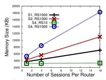
(c) Controller memory needed to keep MultiSpeaker state. S = # of MultiSpeaker per Controller, RS = # of routers per MultiSpeaker.
