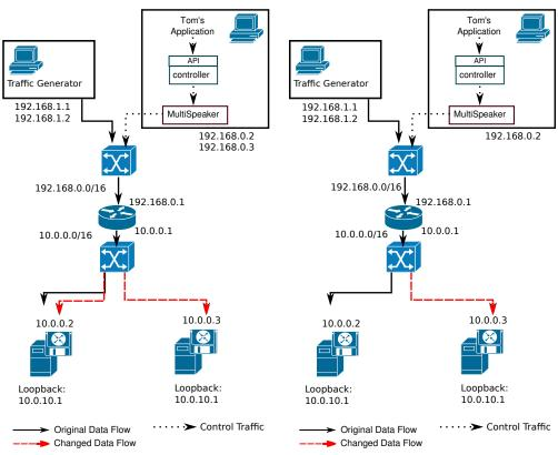
(a) Load balancing scenario setup. The entire RaaS framework is hosted inside a single machine. Unless indicated, addresses are installed on physical interfaces.
