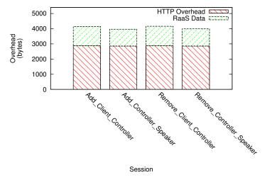
Fig. 6: Network overhead over various operations. x\_y\_z refers to operation x, with caller x and callee z.
