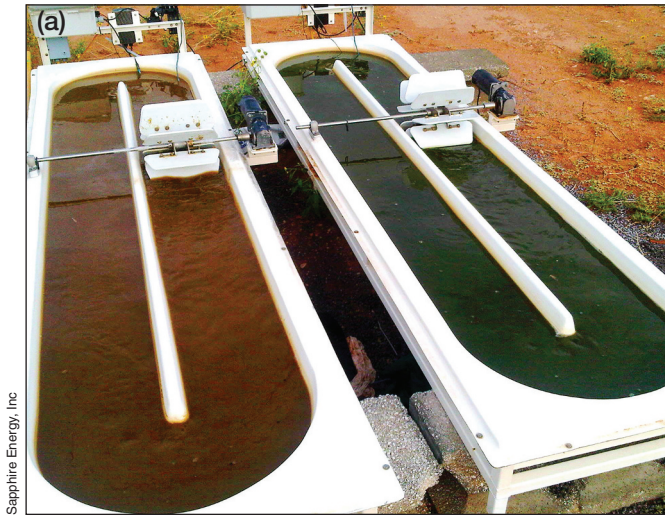
Figure 2. (a) Open mini-ponds operated by Sapphire Energy, Inc. The mini-pond on the left shows the near-total algal crop loss to a chytrid pathogen, whereas the mini-pond on the right illustrates what a productive pond looks like. (b) Both the abundance and diversity of pathogen strains were observed to increase over time in an open raceway pond operated by Sapphire Energy, Inc, using a polymerase chain reaction (PCR) approach. Note: the “cycle threshold number” decreases as fungal pathogen abundance increases. Fungal pest A (blue dots and trendline) is Amoebophilidium protococcarum , and fungal pest B (red dots and trendline) is Amoebophilidium occidentale ; fungal pest C (green dots and trendline) is currently unknown but is genetically distinct from the first two pests.
