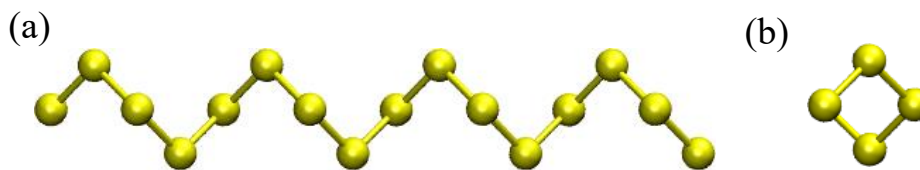
Figure 2.9 Calculated structure for the sulfur helix in S@SWNTs: (a) side-view, (b) cross-sectional view. (Calculation was done by Dr. M. Belén Oviedo from Professor Wong group)
