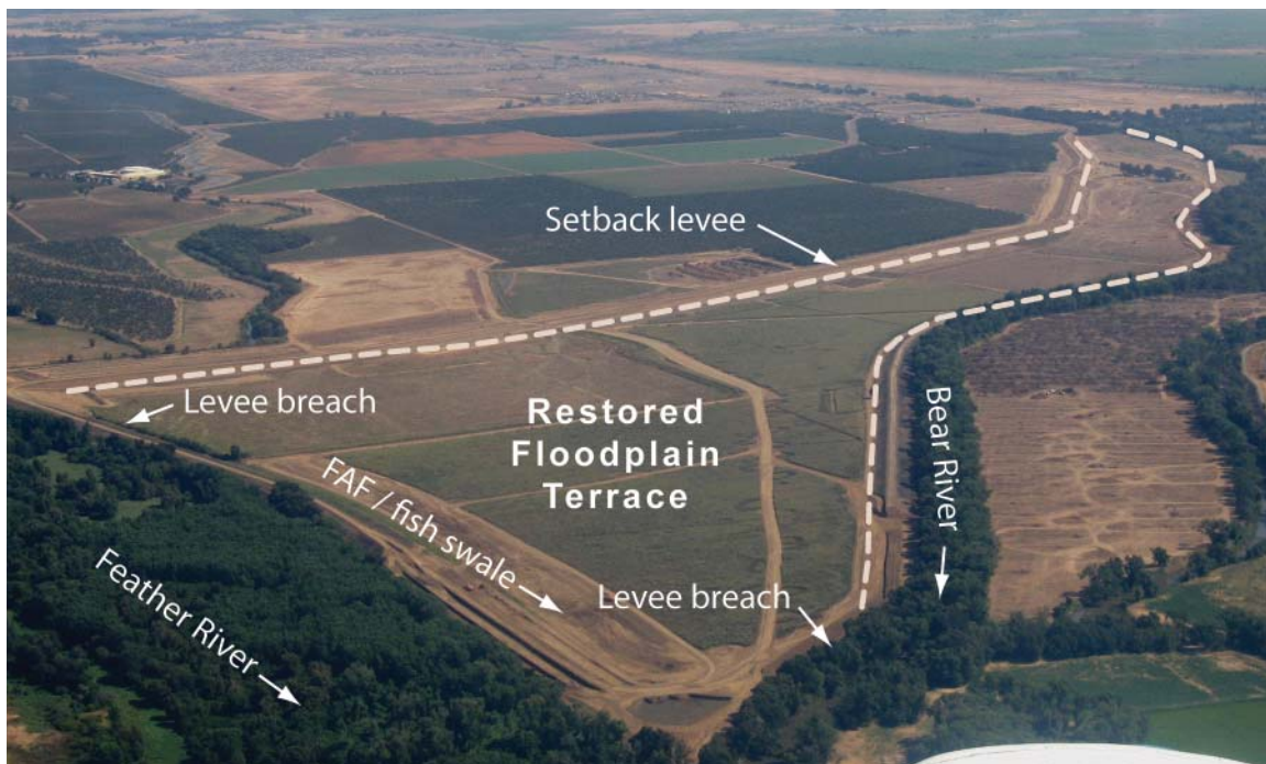
Figure 17 Bear River Levee Setback Project, design based on FAF approach
