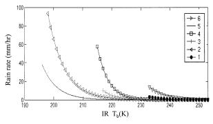
FIG. 6. (a) The calibrated cloud–rainfall relationships (400  $T_b$ –R curves) from the PERSIANN CCS algorithm using IR and radar data, with each curve referring to a cloud cluster in the SOFM classification map (Fig. 5a.). (b) Several typical  $T_b$ –R curves from clusters in (a). Note that the curve of cluster 0 does not show in (b) because it is short and flat.
