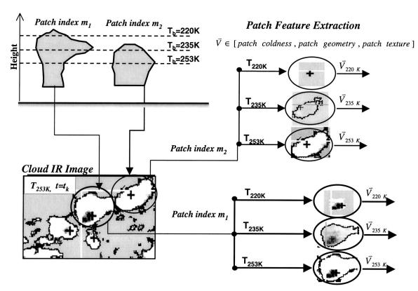
Fig. 4. Cloud-patch features calculated at three separate temperature levels (220, 235, and 253 K).
