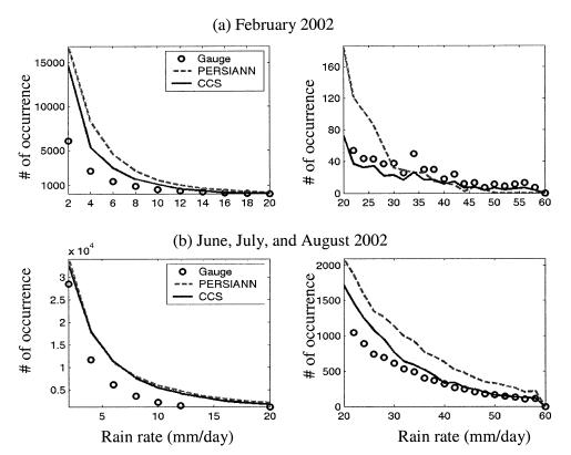
Fig. 13. Plots of rain rates (mm day<sup>-1</sup>) during (a) Feb 2002 and (b) Jun–Aug 2002 for (left) rain rates from 0 to 20 mm day<sup>-1</sup> and (right) rain rates from 20 to 60 mm day<sup>-1</sup>, both in 2 mm day<sup>-1</sup> increments. Numbers on the x axis represent rain-rate boundaries, and numbers on the y axis are the number of rain-rate occurrences. The validation region is the same as in Fig. 12.
