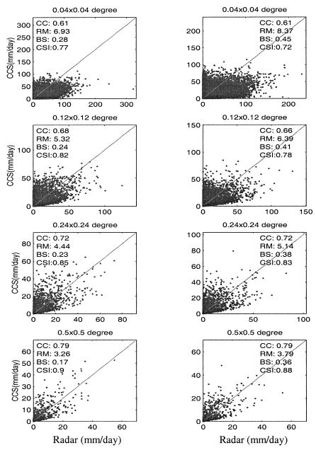
Fig. 8. Scatterplots of radar measurements vs PERSIANN CCS-estimated daily rainfall at four spatial scales for a region located at  $25^{\circ}-45^{\circ}N$ ,  $100^{\circ}-120^{\circ}W$  on (left) 8 Jul and (right) 9 Jul 1999.
