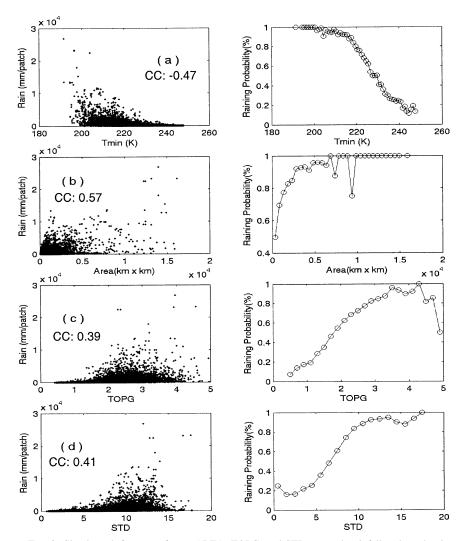
Fig. 3. Cloud-patch features of  $T_{\min}$ , AREA, TOPG, and STD vs patch rainfall and patch rain probability. Note that not all of the selected features are shown here. (left) Values of cloud-patch features vs cloud-patch rainfall, and (right) interval-averaged values of cloud-patch features vs patch rain probability.
