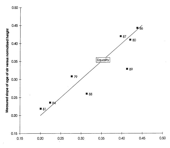
Predicted slope =  $2.59E3 * FlowRate(m^3/s)/Loads(W) + 0.95 * (Archimedes); r^2 = 0.81$  Figure 6. Measured versus predicted slope of age of air versus normalized height. Prediction based upon multiple linear regression with Archimedes number and ratio of supply flow rate to internal heat load as variables. Test numbers shown.
