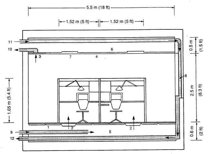
Figure 2. Cross section of CEC. Numbered items are: 1 = floor panel; 2 = TAM; 3 = return grille; 4 = suspended ceiling; 5 = subfloor plenum; 6 = ceiling plenum; 7 = light fixture; 8 = annular space between windows; 9 = air supply to subfloor plenum; 10 = air return to HVAC system; 11 = conditioned air supply to annular space; 12 = air return from annular space to HVAC system. The return-air grille is centered between the front and back walls.
