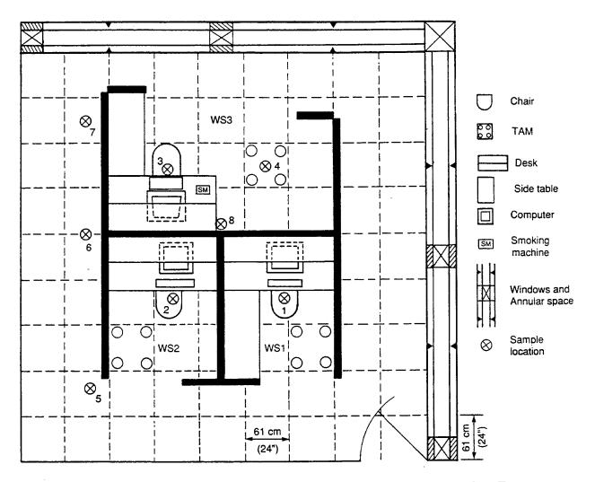
Figure 3. Plan view of CEC with workstations denoted WS1, WS2, and WS3. Tracer gas was sampled at points 1 - 4 (0.4 m, 1.1 m and 2.1 m above floor), and at points 5 & 7 (1.1 m above floor), at point 6 (1.1 m and 2.1 m above floor), and at point 8 (2.1 m above floor). Particles were sampled at points 2 and 3 (1.1 m and 2.1 m above floor).
