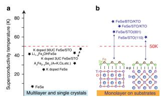
**Figure 4 | Superconductivity temperature of FeSe-related superconductors.** (a) All the multilayer and single crystals of iron-based superconductors show  $T_c$  lower than 50 K. (b) In contrast, monolayer FeSe on various  $TiO_2$  terminated substrates always show  $T_c$  higher than 50 K. We have observed electron-phonon coupling both at FeSe/STO(001) and FeSe/STO(110). The  $T_c$  of FeSe/STO/KTO is from ref. 32.
