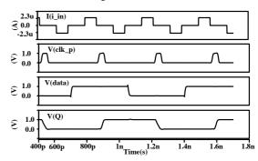
(b) Simulation waveforms confirm the internal current-to-voltage pulse generation (clk\_p) that triggers input data capture.
