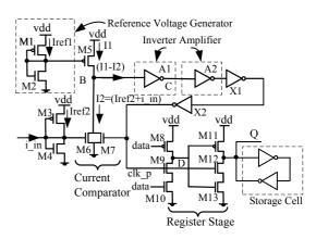
(a) The proposed CMPFF uses current-comparator and feedback connection to generate a voltage pulse that triggers a register stage to store data in the storage cell.
