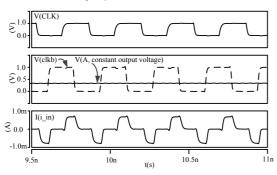
(b) Simulation waveforms confirm a VM input is converted to a constant CDN voltage and a representative push-pull current at each CMPFF.
