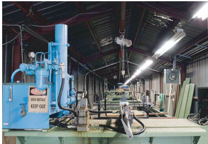
Figure A.4: UC Berkeley Tow Tank facility in Richmond, CA. Schematic (top) and image of the facility with the wavemaker mechanism seen in blue in the foreground (bottom).
