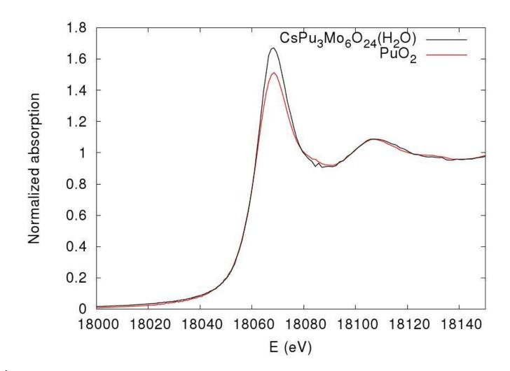
Figure 6. Pu XANES comparing the standard  $Pu(IV)O_2$  to  $CsPu_3Mo_6O_{24}(H_2O)$  indicating that Pu is in the tetravalent state.
