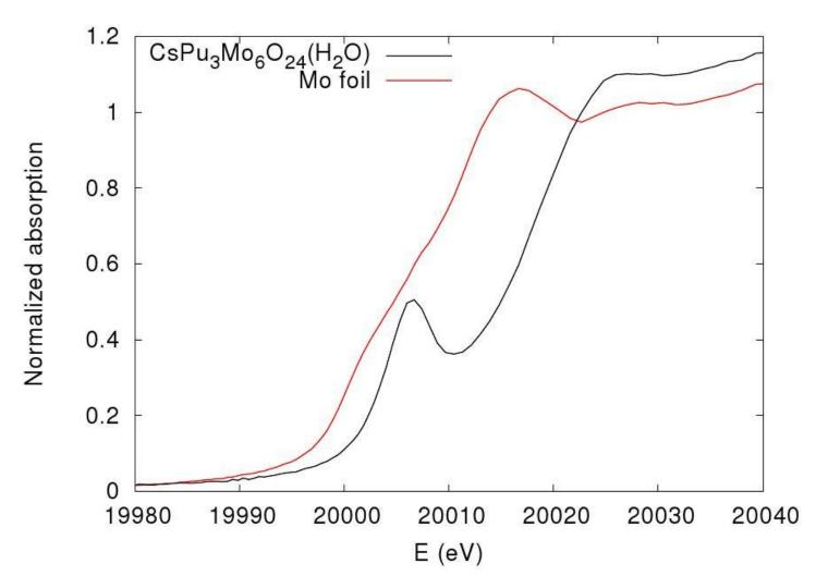
Figure 7. Mo K-edge XANES exhibits a substantial pre-edge absorption peak making analysis difficult however, the energy at half-height of the edge indicates a Mo(V) or Mo(VI) valence.
