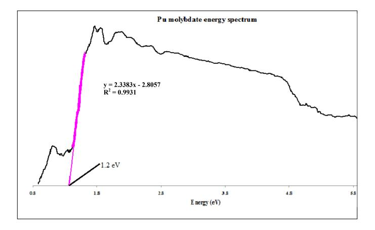
Figure 5. Optical energy spectra of  $CsPu_3Mo_6O_{24}(H_2O)$  used to determine the approximate bandgap. The least squares fit of the highlighted region is shown along with the x-intercept that is the calculated bandgap.
