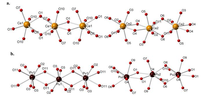
Figure 2. The coordination environments of the Ce(IV) (orange spheres) and Pu(IV) (dark red spheres) metal centers consisting of alternating edge sharing chains. All coordination environments are eight-coordinate square anti-prisms with approximate  $D_{4d}$  symmetry. The chains are linked by molybdate polyhedra to build the framework.
