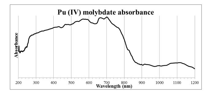
Figure 4. Absorption spectrum of  $CsPu_3Mo_6O_{24}(H_2O)$  showing the strong absorbance from approximately 250 nm to 800 nm. The typical f-f transition analysis fails here since those features are overwhelmed.
