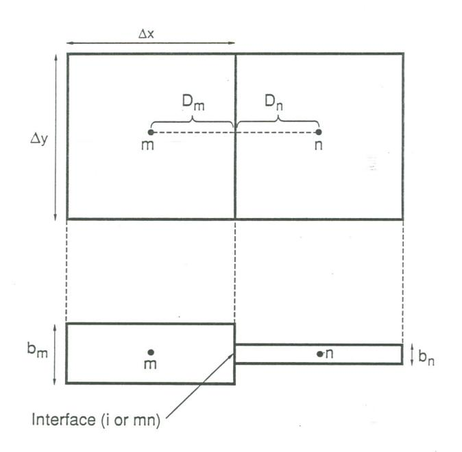
Figure 6. Schematic of a connection between two fracture elements, looking down onto the fracture plane (top), and giving an elevation view (bottom).
