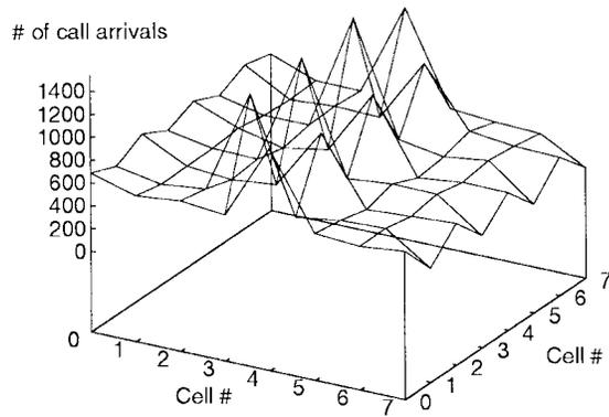
Fig. 4. Load profile (15% imbalance, 27 Erlangs per cell average load).
