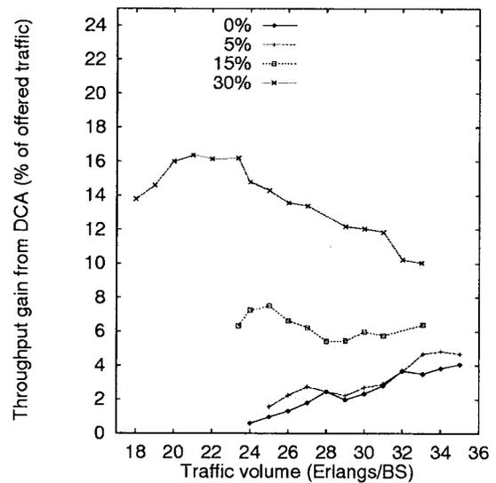
Fig. 12. Average throughput gain from the use of DCA as a percentage of the input traffic.
