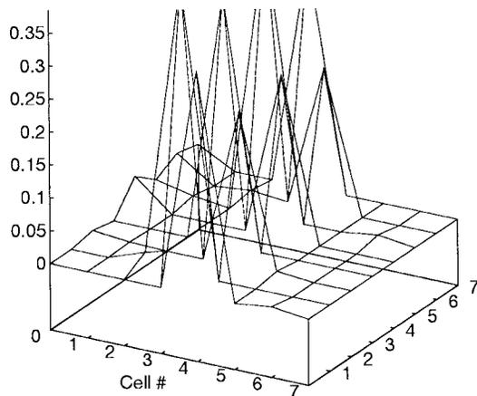
Fig. 6. Blocking probability profile (fixed allocation, 15% imbalance, 27 Erlangs per cell average load).
