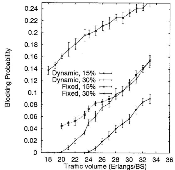
Fig. 3. Blocking probabilities, 95% confidence intervals.
