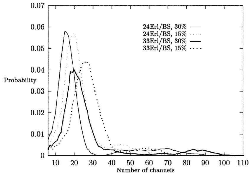
Fig. 13. Probability density of channel utilization at cell, DCA.
