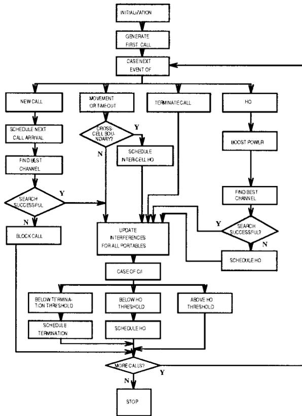
Fig. 2. Simulation model flow diagram.
