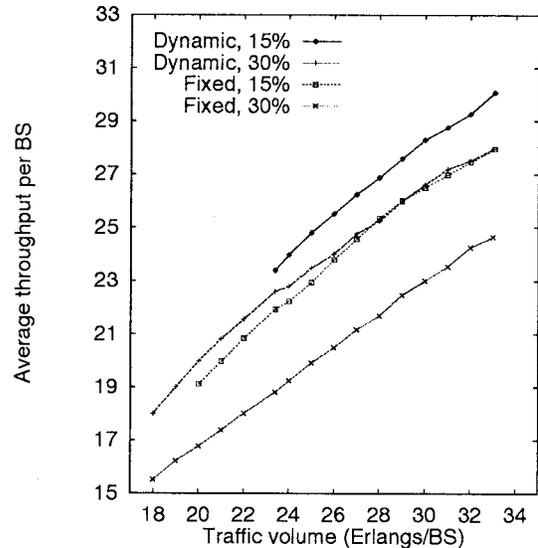
Fig. 11. Average throughput per cell.
