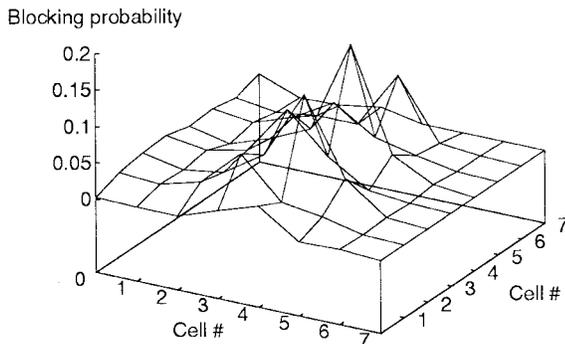
Fig. 5. Blocking probability profile (dynamic allocation, 15% imbalance, 27 Erlangs per cell average load).
