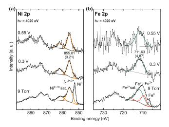
**Figure 3.** Normalized XP spectra of (a) Ni 2p and (b) Fe 2p transitions for a Ni–Fe (7 nm) electrocatalyst, recorded with 4020 eV excitation energy. Bottom to top in (a) and (b): as-prepared catalyst at 9 Torr  $H_2O$  pressure, measurement in 0.1 M KOH at 0.3 V after electrochemical conditioning (6 potential cycles from 0 to 0.65 V), measurement at 0.55 V after additional electrochemical conditioning (6 potential cycles from 0 to 0.85 V).
