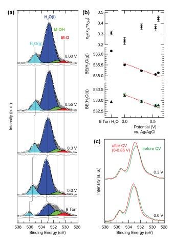
**Figure 2.** (a) Normalized and background-subtracted O1s XP spectra of Ni–Fe (7 nm) electrocatalyst, excited with 4020 eV X-ray photons. Bottom to top: as-prepared catalyst exposed to 9 Torr  $H_2O$  pressure, and operando measurements, taken after extended electrochemical conditioning (6 cycles, 0-0.65 V, and 6 cycles, 0-0.85 V) under a ~30 nm thick 0.1 M KOH liquid film at the indicated applied potentials (vs. Ag/AgCl). The measured spectra (circles) are
