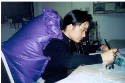
Figure 1. An example of the heating/cooling air sleeve attached to the subject's back.
