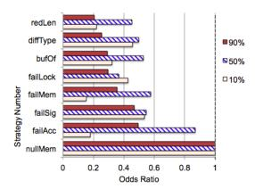
Fig. 4: The impact of perturbation strategies in predicting abnormal program outcome, tested on **all** programs with thresholds of 10%, 50% and 90%. Reference strategy is *nullMem*. Odds ratio shows how much more or less likely a strategy is to cause an abnormal program outcome compared to the reference strategy. Absence of chUid and failNoti means that they are not significant in predicting an abnormal execution.
