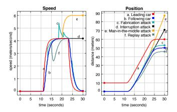
Figure 6: Comparison of Controller behavior under individual attacks
