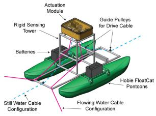
Fig. 1: Aquatic Networked InfoMechanical Systems (NIMS-AQ) prototype craft
