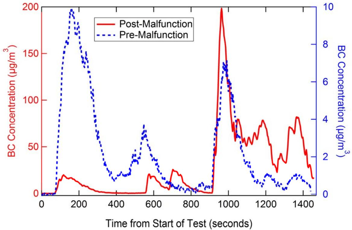
**Figure 3.** Real-time BC concentrations from the Ford Taurus (LEV) during the UC before (Sept. 9<sup>th</sup>; blue line) and after (Sept. 15<sup>th</sup>; red line) malfunctioning. Note the difference in scales for the two axes.
