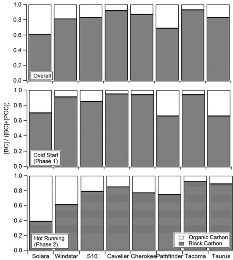
**Figure 4.** Average BC to total carbon (=BC + POC) ratios for LEVs determined from the real-time instrumentation (i.e. PAS and AMS), excluding the days on which non-vehicle BC was added to the SDS.
