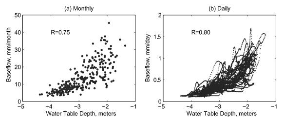
Fig. 4. The (a) monthly and (b) daily scatter plots of the 22-year (1984–2005) baseflow estimated from the daily average streamflow records in Illinois using the digital recursive filter versus observed water table depth.
