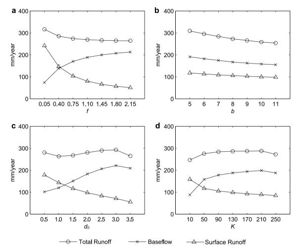
**Fig. 7.** The average annual amounts of total runoff, baseflow, and surface runoff. Each curve represents the average from the 343 runs with only one of the four parameters (*f*,*b*,*d*<sub>0</sub>, and *K*) fixed.
