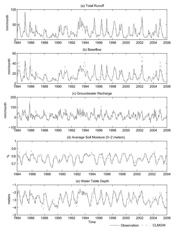
Fig. 5. The 22-year (1984–2005) monthly time series of (a) total runoff, (b) baseflow, (c) groundwater recharge, (d) soil moisture, and (e) water table depth in comparison with observations.
