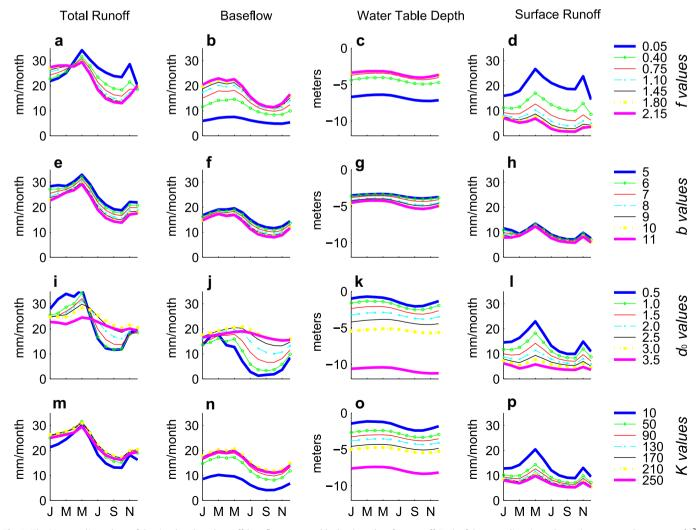
**Fig. 6.** The 22-year climatology of the simulated total runoff, baseflow, water table depth, and surface runoff. Each of the seven lines in each panel represents the average of 7<sup>3</sup> (=343) runs with one of the four calibration parameters fixed at the given value.
