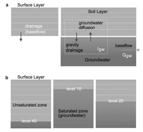
**Fig. 1.** (a) Schematic representation of the soil layer and groundwater model. The left panel is the default CLM without the groundwater model.  $I_{gw}$  is groundwater recharge;  $Q_{gw}$  is groundwater discharge. (b) The flexible soil-layer configuration in the CLMGW structure.
