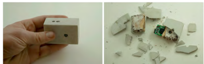
Figure 4. An Inaccessible Digital Camera with a concrete enclosure.
